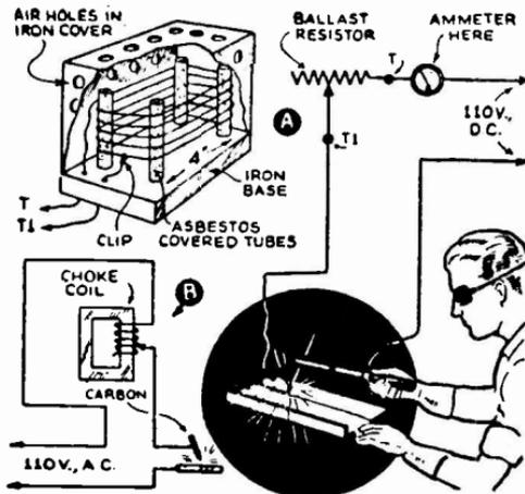
layers of No. 14 D.C.C. copper wire placed on one or both of the longer legs of the core. It is well to bring out taps from each layer after the second, and diagram B shows how the adjustable choke coil is connected in series with the arc.
