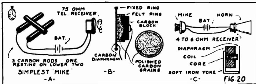
Simple home-made telephone apparatus
