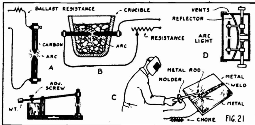
Electric Arc, Furnace and Welder
