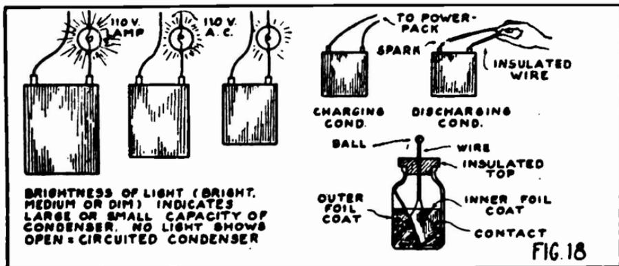
Condenser tests easily made with 110-volt lamp
