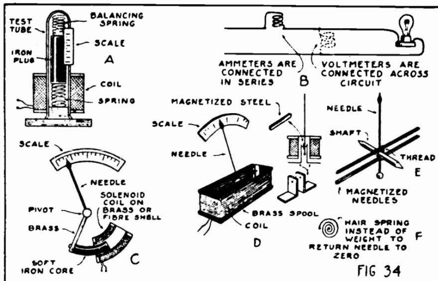
Home-made electrical Measuring Instruments
