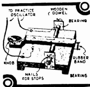
rising too high or otherwise getting into an inconvenient position. Contacts may be made through nails, screws or any other metal driven through the arm and baseboard.
