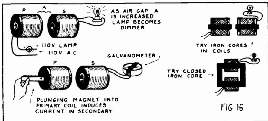
Induction experiments — iron cores intensify the results
