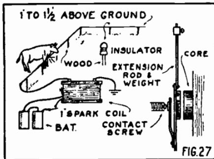
Electric fence shocker — it saves miles of wire and hours of time
