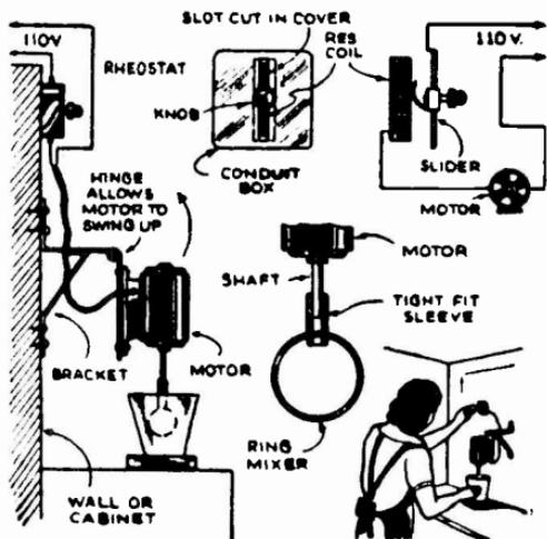
Variable speed mixer mounts on wall or cabinet, and can be used for stirring drinks or batter, whipping cream and other kitchen tasks
