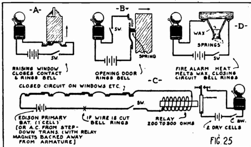
Burglar alarm circuits, including a closed circuit; if wire is cut, bell rings
