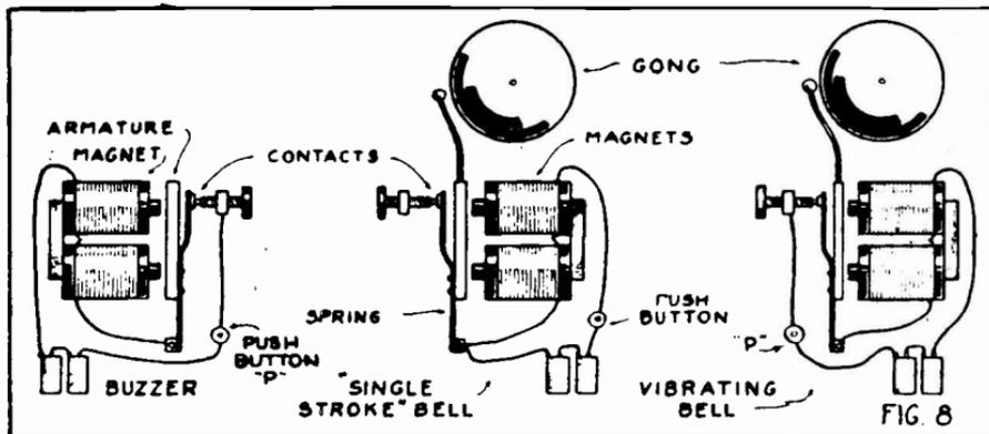
A buzzer — a single-stroke bell and a vibrating bell
